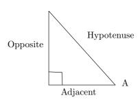
The third side, the side between our angle and the right angle is called the adjacent side. It is important to remember that the opposite and adjacent sides are named in relationship to the angle A or the angle we are using in a problem. If the angle had been the top angle, the opposite and adjacent sides would have been switched.
